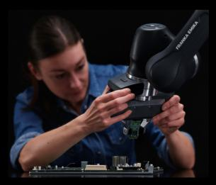
C. Teach the robot by manual guidance and parameterize each App via dialog-based interaction.
